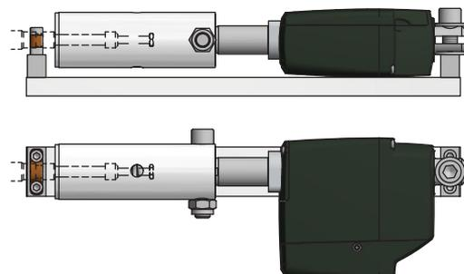
All our painter hooks can be used together with the Integrated Henriksen System (IHS), which eliminates the possibility of opening the painter hook before the main hook.
