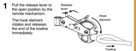
2 When the hook element has released the towline, let the release lever go. R
