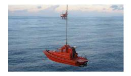
Using a swivel joint allows the lifting arrangement to pivot and reduces the risk for a lot of potential unwanted loads. We recommend always using a swivel, especially for boats that are frequently used.
