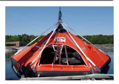
If conditions are such that it is not possible to use the automatic release capability, the Henriksen Liferaft Hook also offers a manual opening facility. It can be used if the raft is on the water but is being pulled by a strong current or by vessel movement and the automatic release capacity is not enough. Under these circumstances, a green grip on the hook can be pulled strongly and the hook will open.
