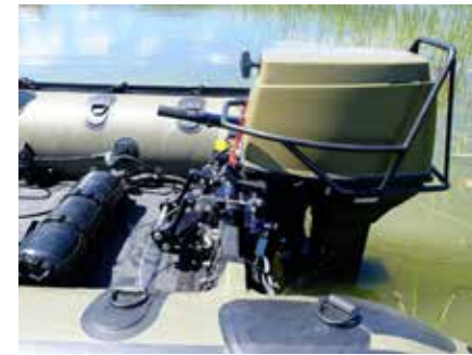
UNDERWAY CONFIGURATION OBM is locked in the operational/down position. The OBMs full range of trim, steering & shallow water drive settings still available.
