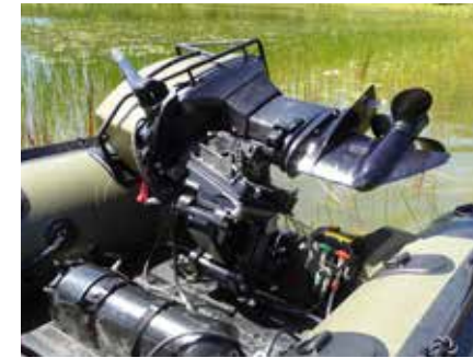
STOWED CONFIGURATION Obm is locked above and parallel to transom.
