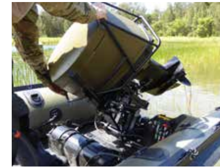
RAISED CONFIGURATION OBM is locked above and perpendicular to transom. OBM is retained by a single pin. Once removed, the OBM slides out of the bracket for quick and safe changeout at sea.
