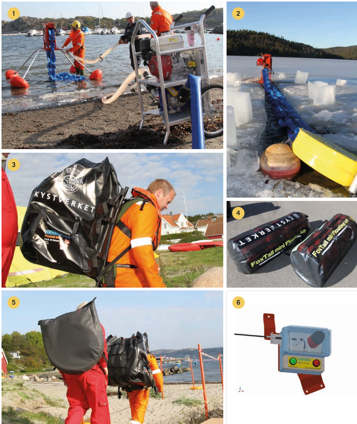
1. FoxPump, special designed that also can tackle heavy oil. 6 m 3 /h, 9 bar, 2. Floating pulley, 3. Backpack (can be carried of one or two people), 4. Floating kit with bag, 5. Extra set of hoses in bag (5m suction and pressure), 6. Wireless remote control
