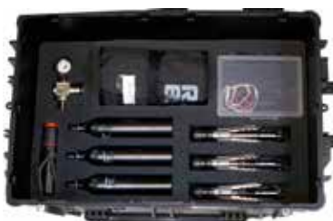
Spareparts, Grapnels, Maintenance Box and Fill Line Valve are below the bag in the box.
