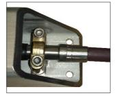
7 Set a washer and the nut right on the cable end. Do not tighten yet.
