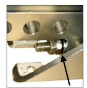
**18** Make sure that there is small gap between the release handle and the upper part of the latch, refer to the illustration. Adjust the position of the fork and the nut on the cable if necessary.
