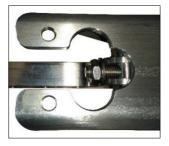
8 Spray a small amount of lubricant oil into the remote unit.
